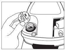
**Step 3** Check oil level. Oil level should always be between the "FULL" and "ADD" marks on the dipstick. Be sure the machine is level when checking the oil level. (Refer to the engine's operating manual for seasonal grades.)
